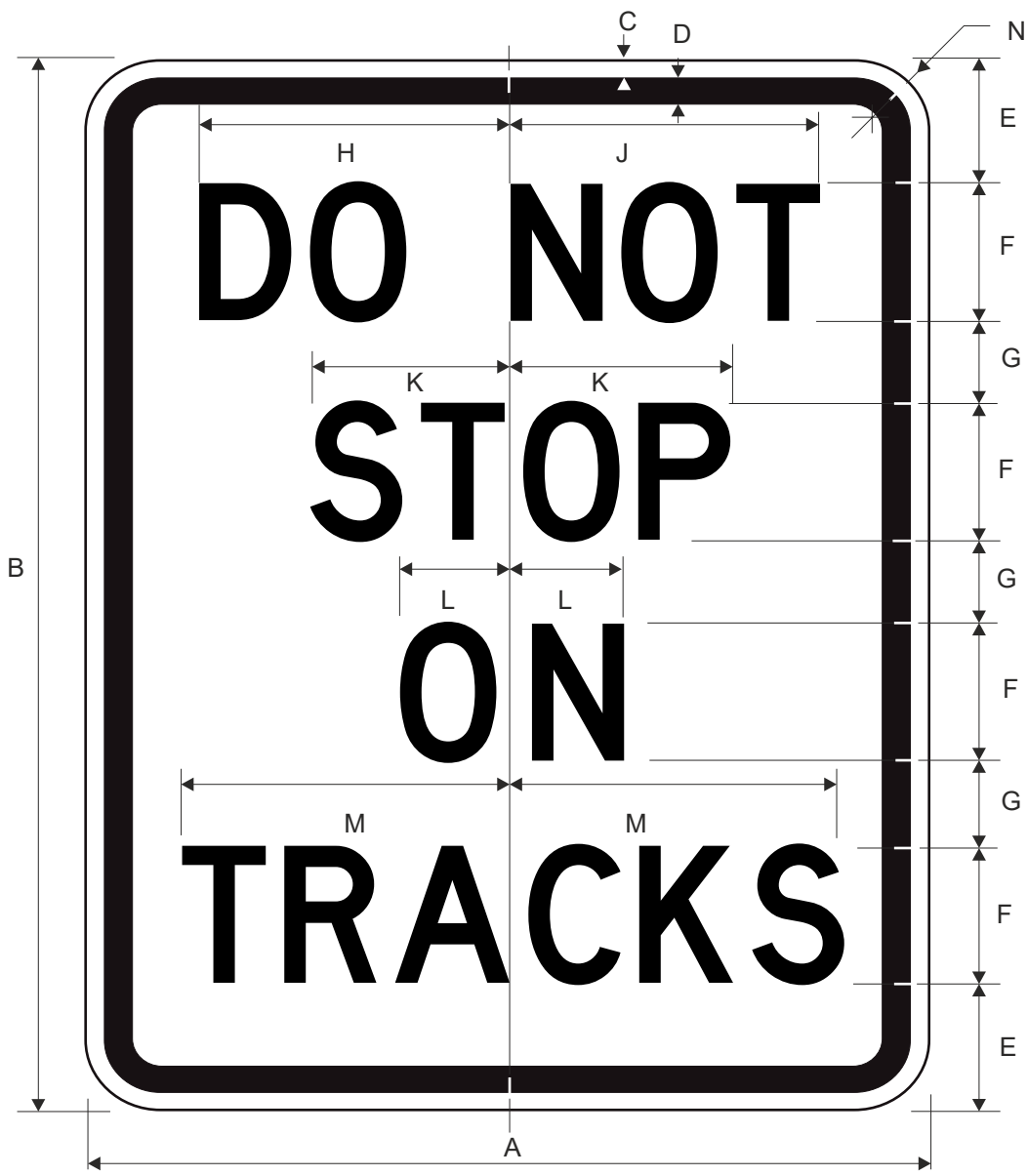
R8-8 DO NOT STOP ON TRACKS
