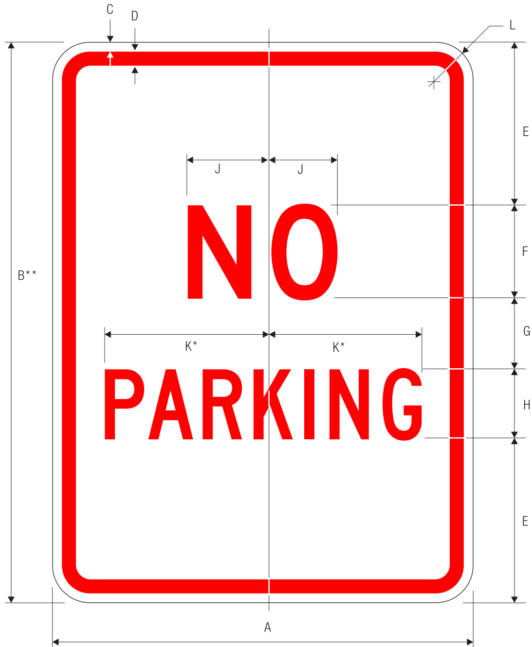
R8-3a NO PARKING *Reduce spacing 50% for 24", 36" & 48" sizes. **Recommend square shape for 36" and 48" sizes.
