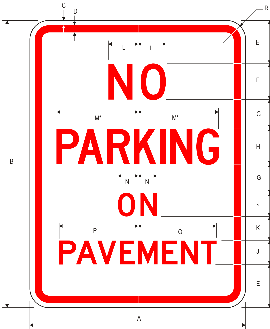
R8-1 NO PARKING ON PAVEMENT
