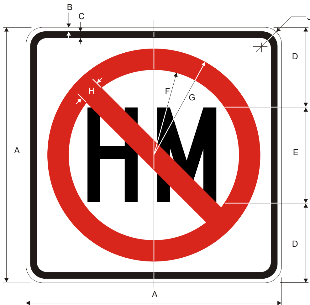
R14-3 No Hazardous Material
