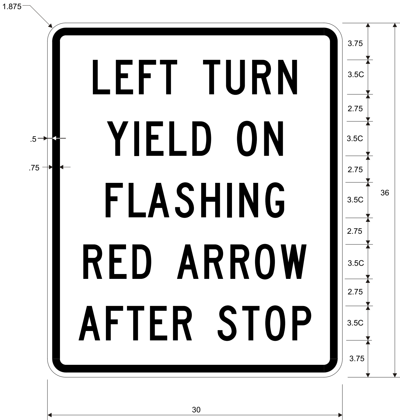
R10-27 LEFT TURN YIELD ON FLASHING RED ARROW AFTER STOP
