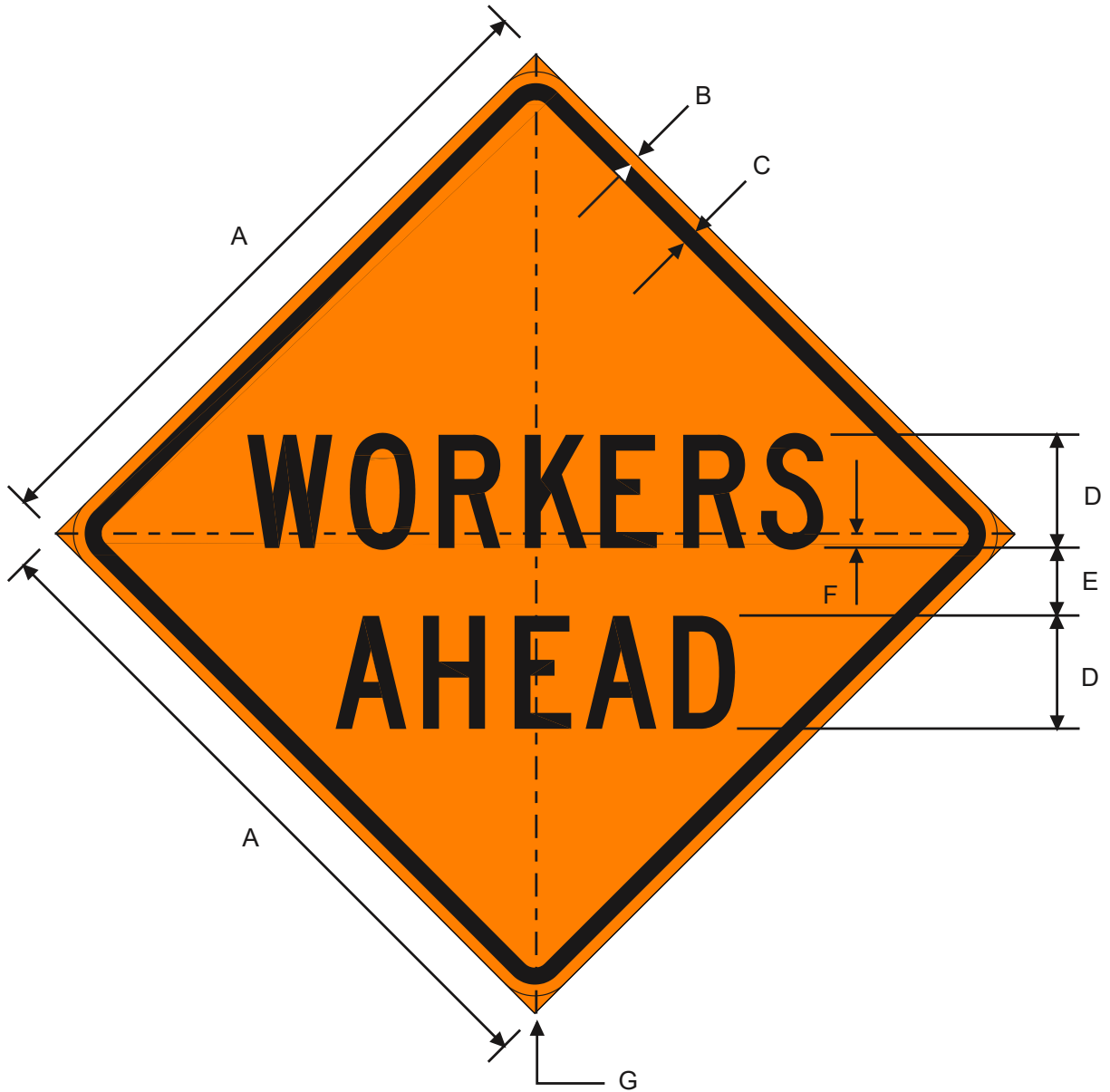
CW21-1bT WORKERS AHEAD
