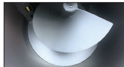
Oversized 14" auger with bottom bead sweep
