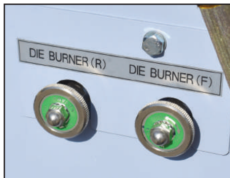
Operator located die burner controls
