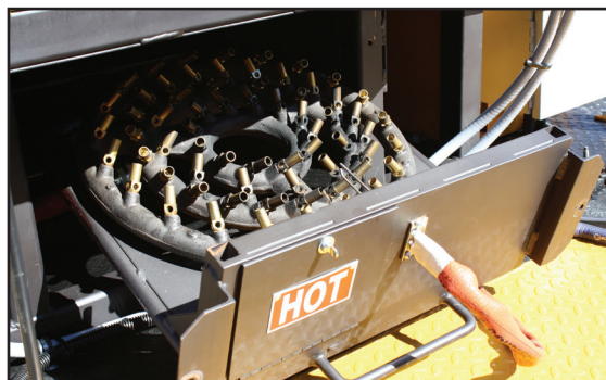
Burner ring slides out on rack, allowing for easy service of jet burners.
