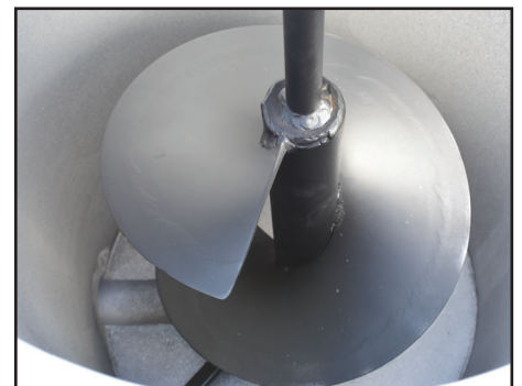
14" Auger agitation with bottom blade
