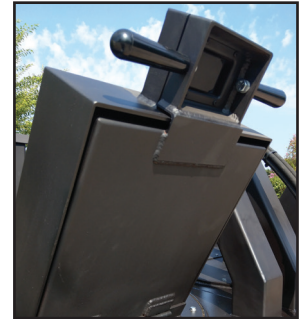
Flash-safe material feed doors are designed to prevent injury to operator.
