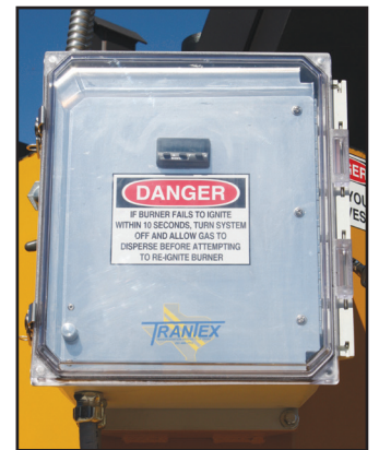
Digital Thermostats with automatic spark ignition systems allowing burners to be ignited with a simple toggle switch.
