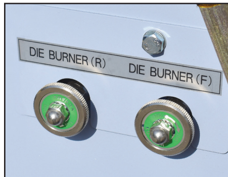
Operator located die burner controls
