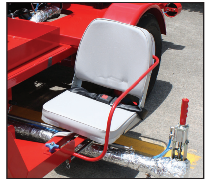
Quick release to fold up for easy transporting
