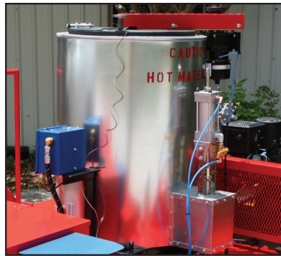
Efficiently heated tank by a 60,000 BTU burner
