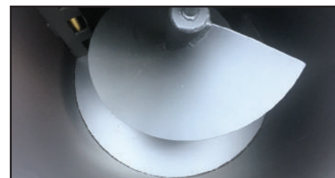
Oversized 14" auger with bottom bead sweep
