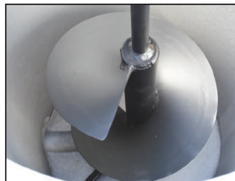
14" Auger agitation with bottom blade
