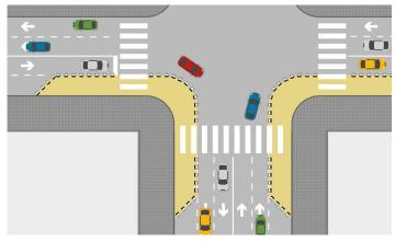
WIDENING OF THE SIDEWALKS AND NARROWING OF THE STREETS AT INTERSECTIONS. Easily creates safe intersections.
