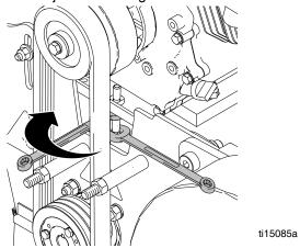
3. Use two wrenches to loosen motor mount bolts on each side of scarifier base.
