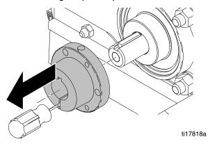
4. Remove all four nuts holding drive side bearing onto cage.
