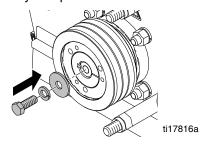
4. Install sheave onto bushing and evenly tighten the three bolts and lock washers to pull the sheave onto the bushing.
