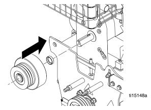
2. Use impact wrench to tighten clutch bolt.
