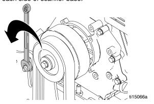
4. Tighten bottom bolt to lower pulley plate.
