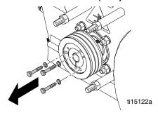
4. Insert the three bolts into the pulley removal holes. Evenly tighten the screws to slowly remove pulley.
