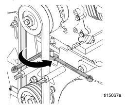
5. Replace belt shroud and tighten three nuts and four screws.
