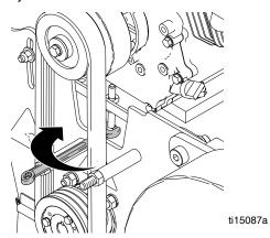
3. Tighten belt adjustment bolt according to recommended tension below.
