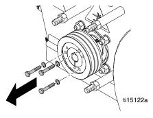
Insert the three bolts into adjacent removal holes and evenly tighten to remove sheave from bushing.
