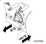
5. Slide shaft assembly out of holes.
