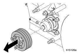
d. Remove set screw from bushing.
