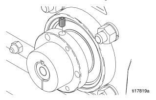
e. Remove bushing from drive shaft. If bushing is very tight, tap a flat-head screwdriver into slot on bushing to open it up and slide off shaft.
