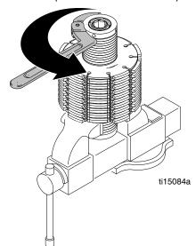
3. Remove drum from vise and install drum (see **Drum Replacement**, page 7).
