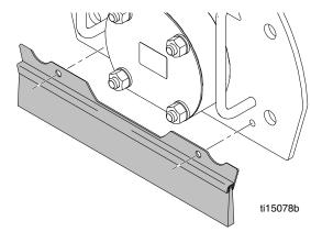
2. Tighten two mounting bolts.
