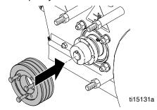
7. Insert three pulley bolts and washers.
