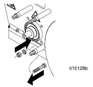
3. Make sure drive shaft key is assembled as shown below.
