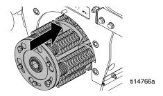
Non-DCS Models: Lower Drum Adjustment Dial (D) and pull Drum Engage Lever (E) so drum rests on ground and the door pin lines up with the hole.
