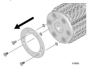
3. Push rod out and remove cutters.
