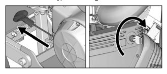
e. After engine starts, move choke to open.
