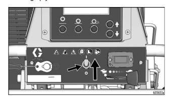
5. **Non-DCS Models:** Rotate Drum Adjustment Dial counterclockwise until a hard stop is felt.
