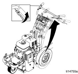
Non-DCS Models: Rotate Drum Adjustment Dial until drum comes into contact with surface and desired depth is reached.
