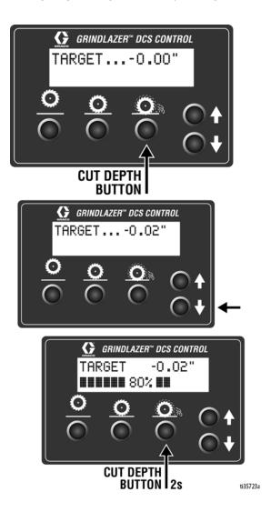
The DCS Control is now ready to grind/scarify. Long press down on the Handlebar Rocker Switch to lower the drum to your Cut Depth Target. Short press up or down on the switch to adjust your Cut Depth on the fly. When finished with your cut, long press up on the switch to raise the drum to the Home position.
