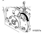
6. Non-DCS Models:Turn Drum Adjustment Dial (D) to maximum height.
