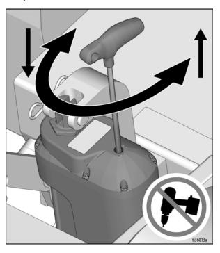
4. Once the desired depth is achieved, replace the screw plug in order to keep water and dust out.
