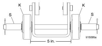
To make a **10 in. cut**, install two spacers (S) on **inside** of Depth Control Wheels (K).
