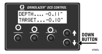
**Long Press:** Lowers the drum to Cut Depth Target.
