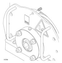
5. Tighten four bolts on Drum Access Panel (H).
