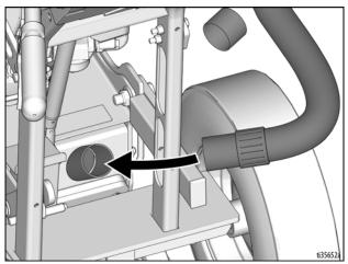
2. Attach vacuum hose to the Inlet Port on the Cyclone Separator (optional) and/or vacuum.
