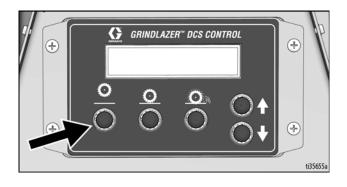
6. **25M994 Model Only:** Make sure Power Switch (B) is in UP position.
