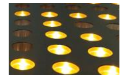
Individual cones for each LED
