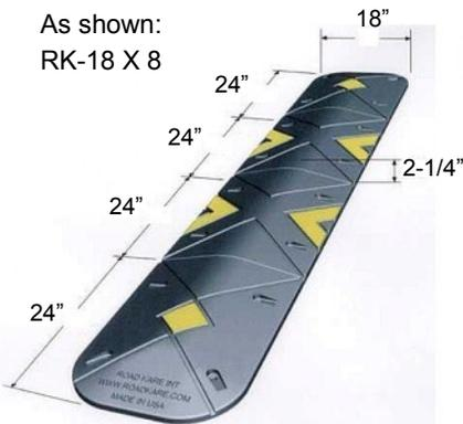
**RK-18** Designed to reduce vehicle speeds to 10 - 15 mph
