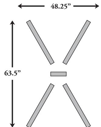
**For maximum wind resistance:** All four (4) legs must be in the down and locked position when using either 36" x 36" or 48" x 48" roll-up signs
